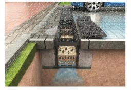
d. Permeable surfaces (infiltration only)
